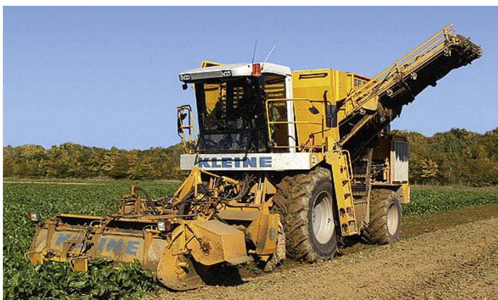
Figure 19: Self propelled 6 row harvester, source: Beet tech Project
